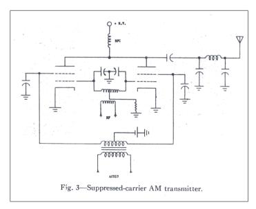
Note that the modulating of carrier frequency of the first pair of balanced modulators is the
