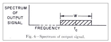
This method of single-sideband generation does not need either sharp cutoff filters or wideband 90 °phase-difference networks. Imperfections in the phasing or balancing do not result in the presence of the unwanted sideband in its usual location. Instead, the unwanted sideband occupies the same band of frequencies as the desired sideband, except that it is inverted. This is a very useful property of this system when channel conservation is an important reason for using single-sideband signals.
