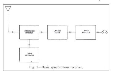
Inspite of the simplicity of this type of receiver, there are several important advantages worthy of note. To begin with, no IF system is employed which eliminates completely the problem of image responses. The opportunity to effectively use post-detector filtering allows extreme
